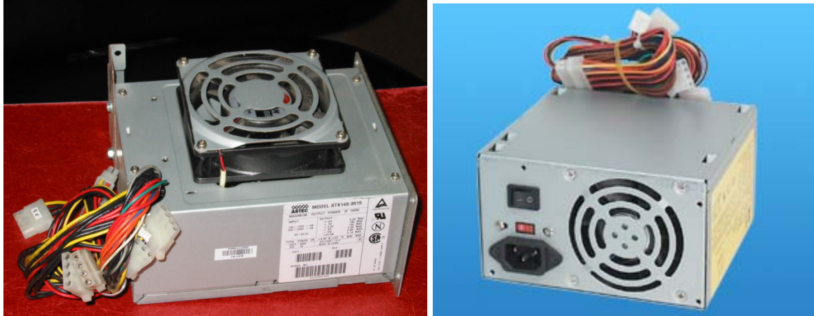
(a) Enclosed Frame Internal Power Supplies
