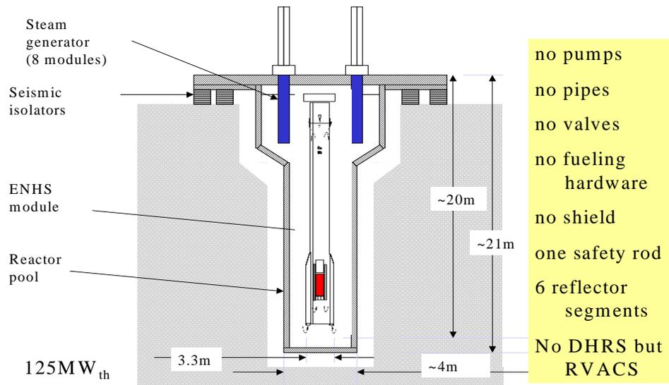
**Fig. 4 General Layout of the Nuclear Steam Supply System of a Power Plant
