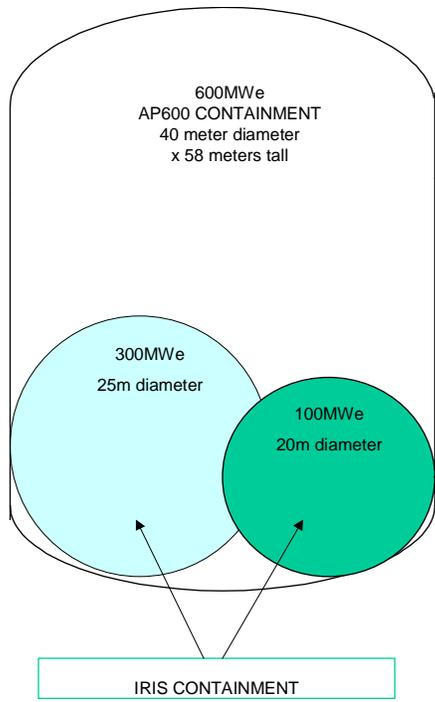
**Fig. 1 Comparison of IRIS Containment
