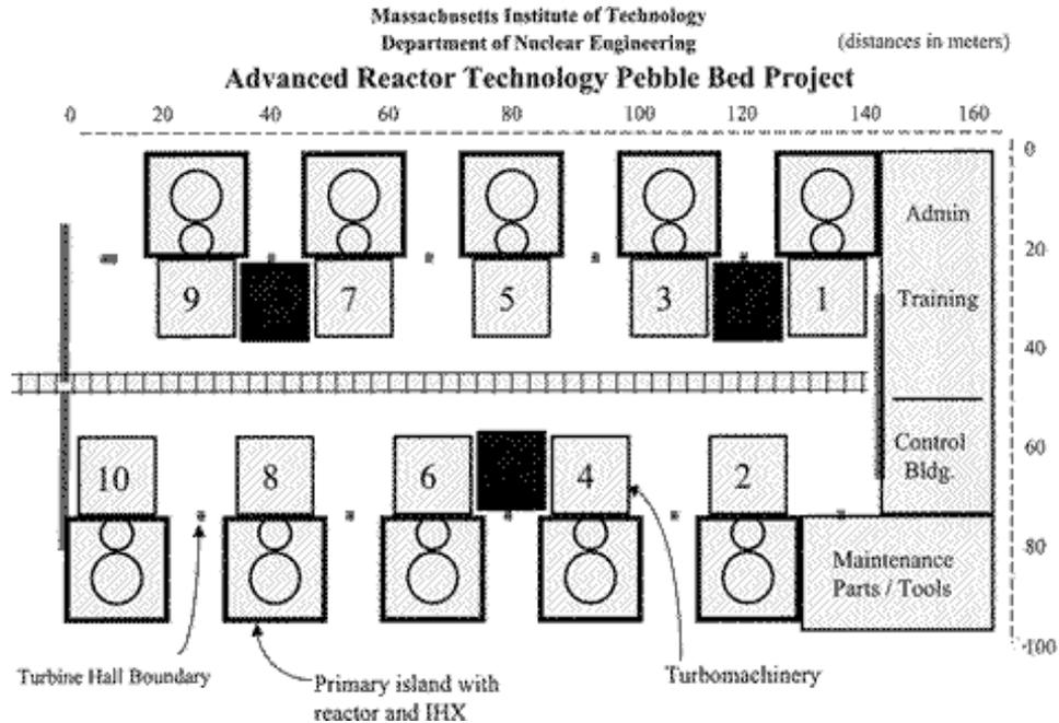
**Fig. 7 A Schematic Layout of a 10-Unit PBMR Power Plant
