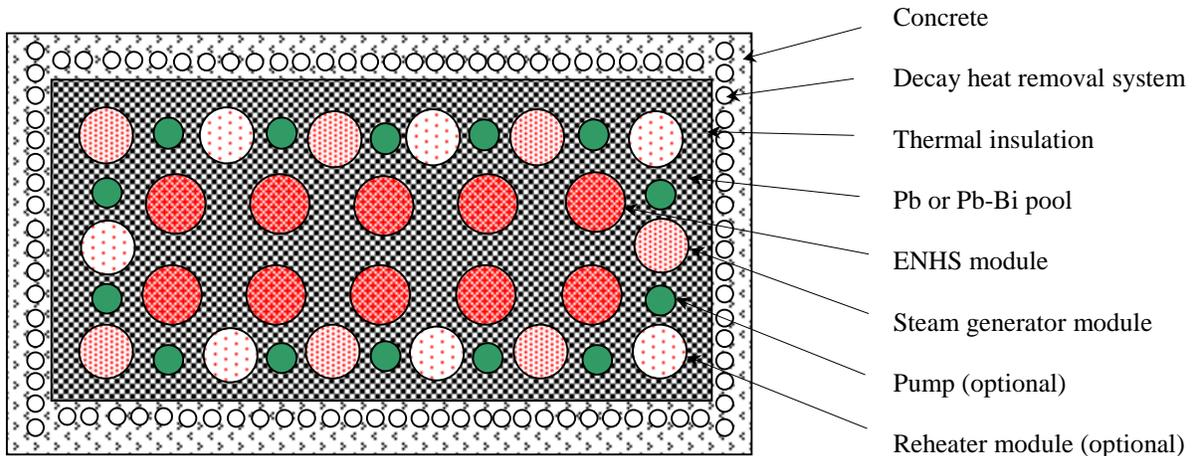
**Fig. 8 A Schematic Horizontal View of a 10-ENHS Module Reactor Using Insulated Concrete Massive Structure for the Secondary Coolant Pool**
