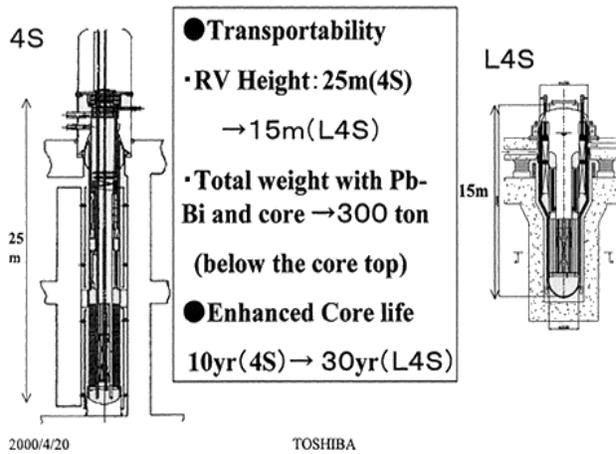
**Fig. 3 Comparison of L4S and 4S Reactors.**
