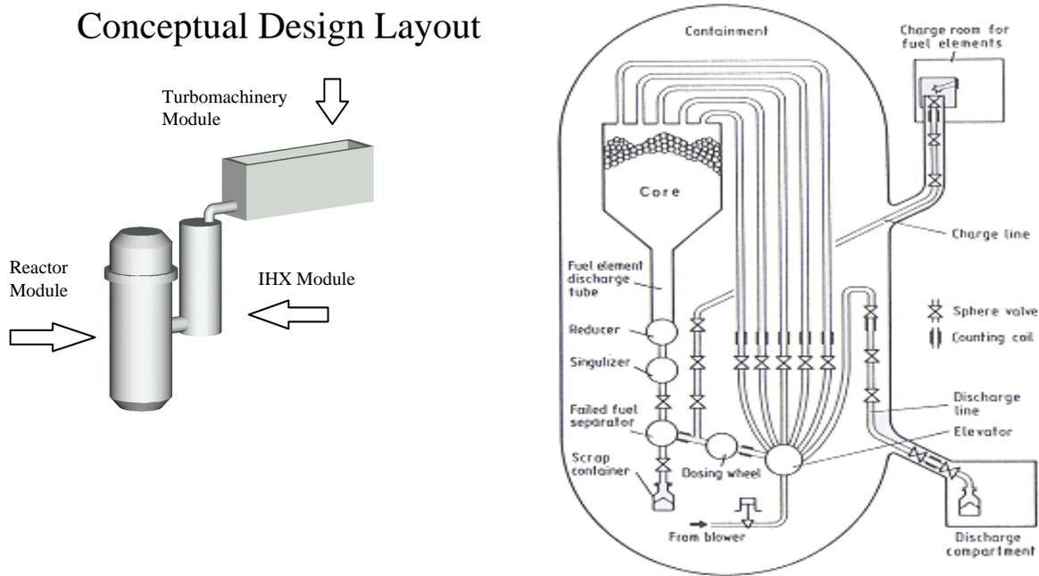
**Fig. 6 Conceptual Design Layout of the MIT Indirect-Cycle PBMR (left) and of its On-Line Fuelling System (right)**<sup>17</sup>
