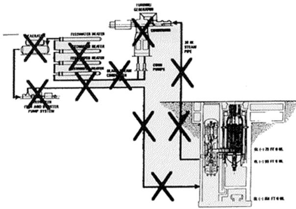
**Fig. 2 The Gas-Turbine Modular Helium-Cooled Reactor (GT-MHR) Plant Schematics Versus Plant Schematic of the Modular High Temperature Gas-Cooled Reactor (MHTGR) that used the same reactor but a steam-driven Rankine, rather than a gas-driven Brayton energy conversion system.<sup>15</sup>**
